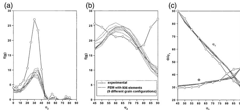
Fig. 5. Set of 9 crystal plasticity finite element simulations conducted by statistically varying the arrangement of the grains in a polycrystalline aggregate. Each grain is represented by 8 integration points and has different neighbor grains in each simulation. (a)  $\alpha$ -fiber, (b)  $\beta$ -skeleton line, (c) coordinates of  $\beta$ -skeleton line.
