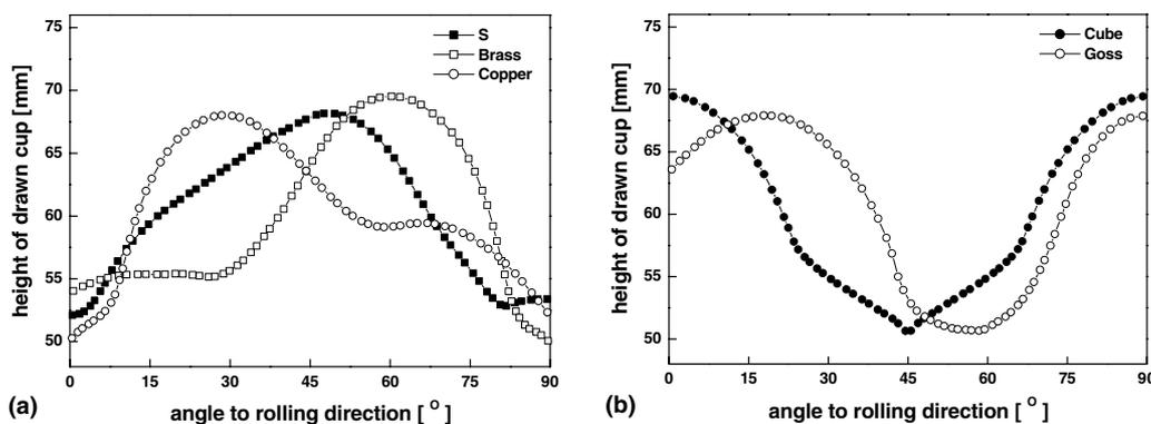
Fig. 5. Ear profiles of individual texture components. Five texture components are selected and their final ear profiles can be grouped into two types (a)  $45^\circ/135^\circ$  type, such as S, Brass and Copper whose main ear peaks appear near  $45^\circ$  and  $135^\circ$  to the rolling direction, and (b)  $0^\circ/90^\circ$  type, such as Cube and Goss, whose ear peaks appear near the rolling and transverse directions.
