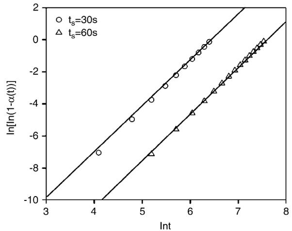
Fig. 6. Avrami analysis: effect of shearing time ( $t_s$ ) at constant time of induction ( $t_0 = 0$  s) and under a constant shear rate of  $1 \text{ s}^{-1}$  during iPP crystallization at an isothermal crystallization temperature of  $T_c = 409$  K.
