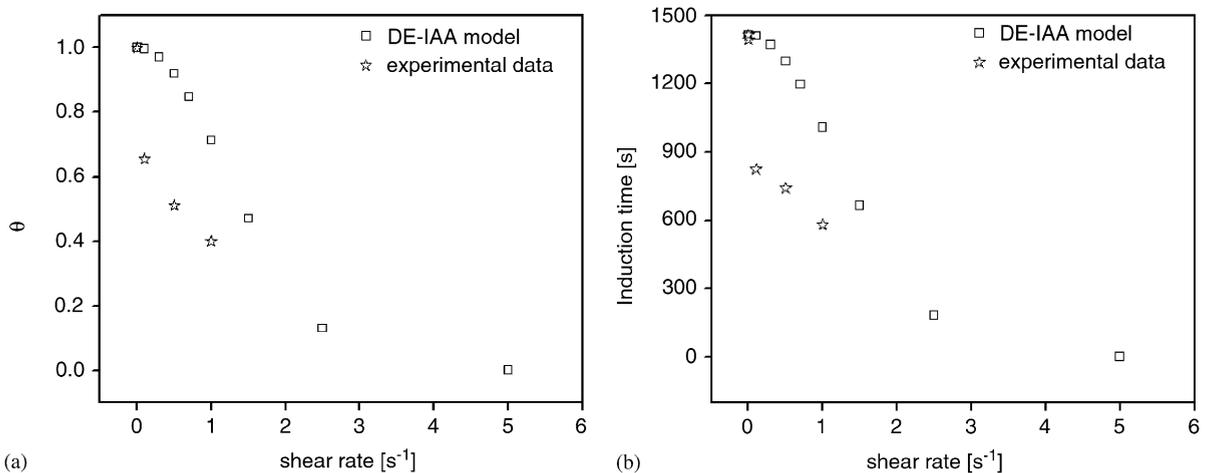
Fig. 8. Dimensionless induction time and induction time as a function of shear rate for iPP at isothermal  $T_c = 409$  K. (a) Dimensionless induction time. (b) Induction time.
