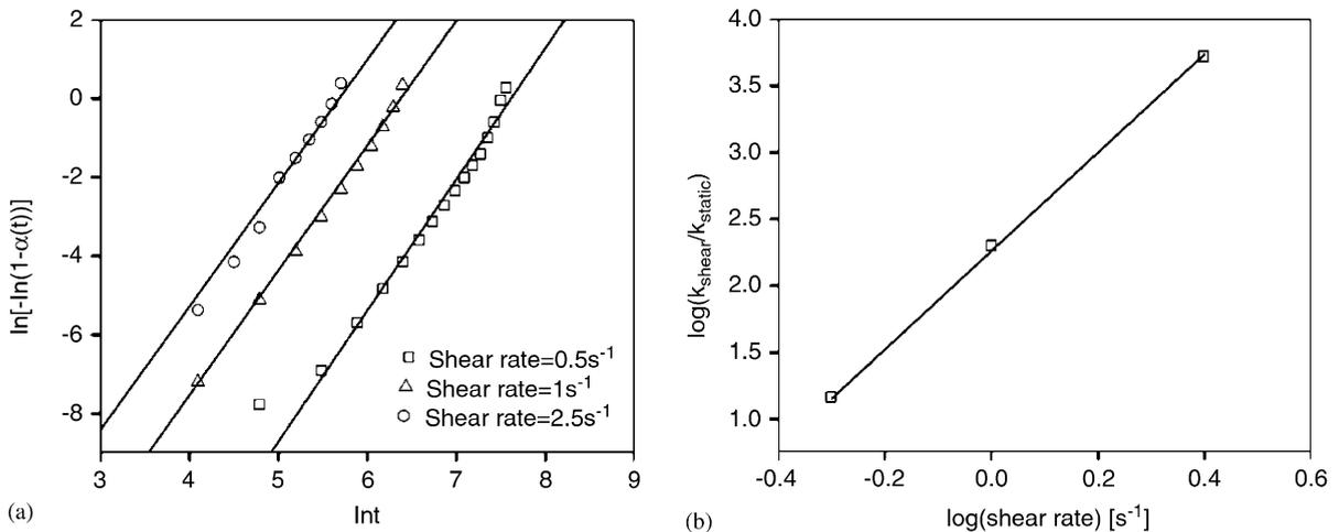
Fig. 4. Avrami analysis: (a) Effect of shear rate at constant shearing time ( $t_s = 30$  s) and induction time ( $t_0 = 0$ ). (b) Relationship between the kinetic rate constants,  $k_{\text{shear}}/k_{\text{static}}$ , as a function of the shear rate for iPP under isothermal conditions at  $T_c = 409$  K.
