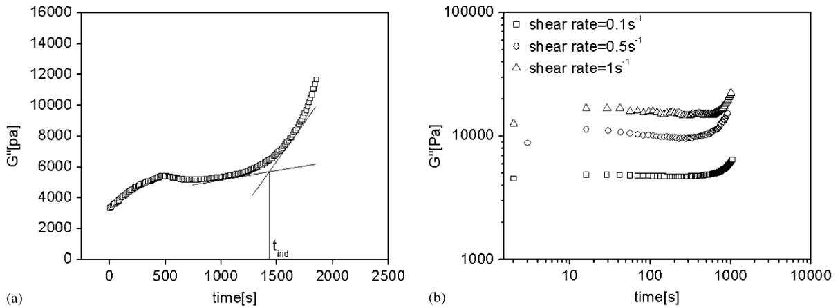
Fig. 7. Effect of shear rate on development of loss modulus at constant shearing time of ( $t_s = 60$  s) and induction time ( $t_0 = 0$ ) for iPP at isothermal  $T_c = 409$  K. (a) Quiescent crystallization. (b) Under shear. Tangent is drawn to determine  $t_{ind}$  (solid lines).
