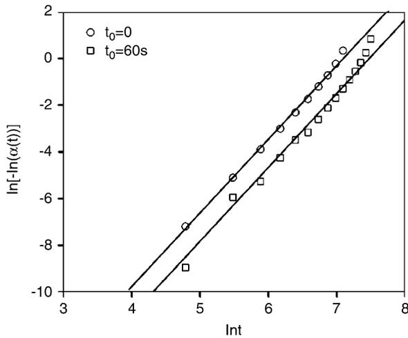
Fig. 5. Avrami analysis: effect of induction time ( $t_0$ ) at constant shearing time ( $t_s = 30$  s) and under a constant shear rate of  $1 \text{ s}^{-1}$  during iPP crystallization at an isothermal crystallization temperature of  $T_c = 409$  K.
