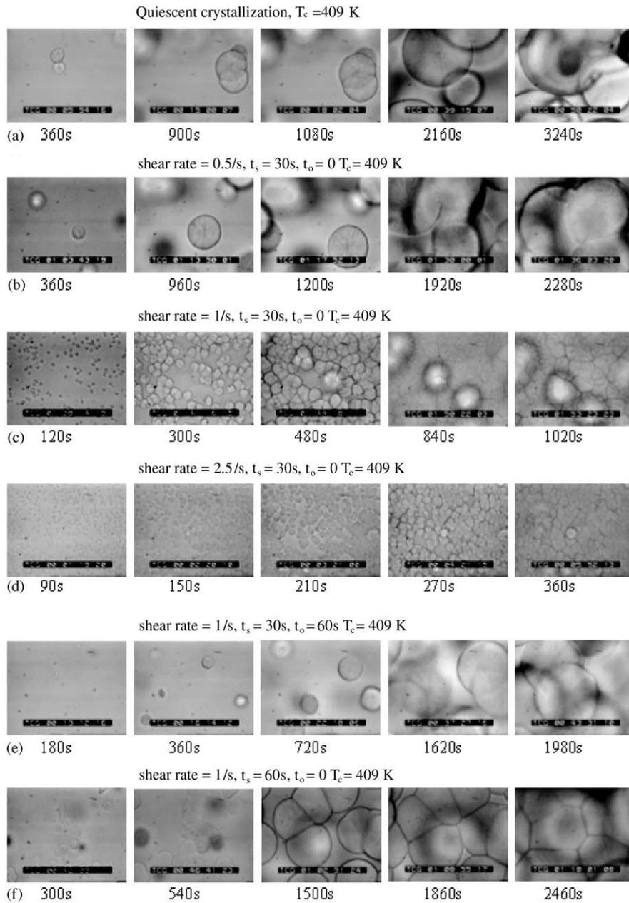
Fig. 2. Optical micrographs taken during the crystallization process after various quiescent and shear treatments (micrograph size:  $240 \times 180 \mu\text{m}^2$ ).
