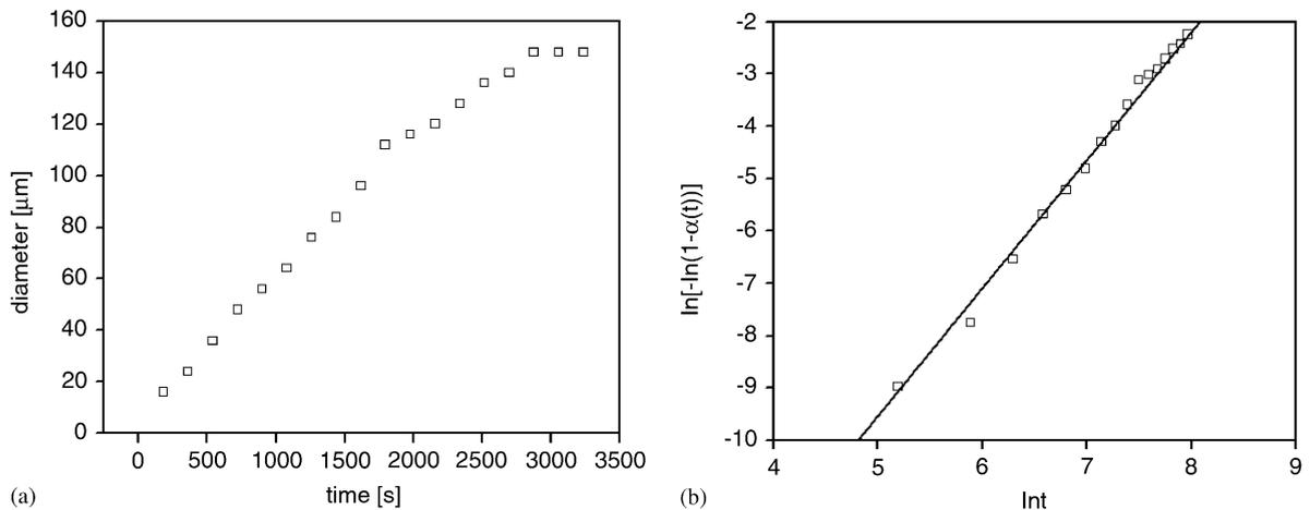
Fig. 3. (a) Quiescent crystallization of iPP at isothermal crystallization temperature 409 K. (b) Avrami analysis applied to the data shown in Fig. 3a.
