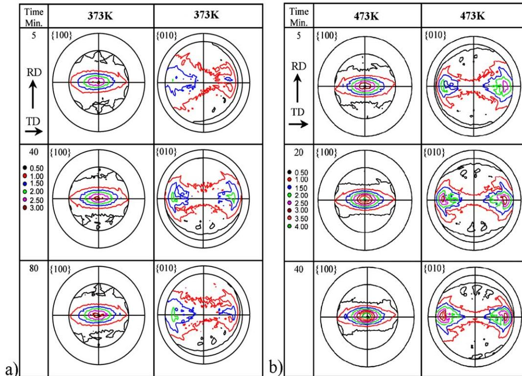
Fig. 6. Texture evolution in terms of pole figures of rolled ( $\phi=1.2$ ) and subsequently heat treated PET. (a) 373 K (b) 473 K. When compared to the rolling textures shown in Fig. 1 the annealing textures are much sharper but not principally different.
