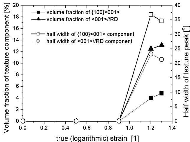
Fig. 3. Development of the crystallographic texture in terms of the volume fractions and spherical half widths of the two main orientation components during rolling. The data were calculated by use of the texture component method from the pole figures shown in Fig. 1. The volume fraction of both components increases, i.e. the texture becomes more pronounced during room temperature rolling.
