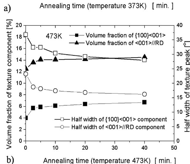
Fig. 7. Changes in the texture components during heat treatment. (a) 373 K, (b) 473 K.
