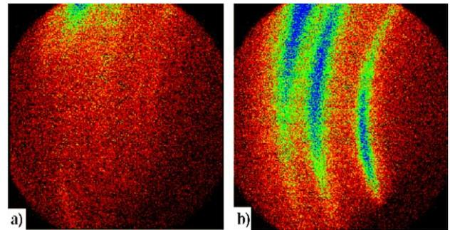
Fig. 4. Debye–Scherrer frames taken for two different tilting angles,  $\phi$ . The different patterns reveal qualitatively how strongly the diffraction data depend on the position of the measurement on the pole sphere. This means that the measurement of the degree of crystallinity cannot be made by simple  $\theta - 2\theta$  X-ray wide angle line scans. Such analysis must in principle take texture into account. (a)  $\phi = 0^\circ$  (b)  $\phi = 90^\circ$ .
