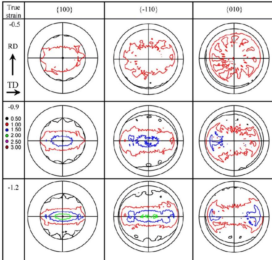
Fig. 1. Experimental pole figures obtained from Debye–Scherrer images for rolled PET (triclinic crystal structure). Rolling was carried out at room temperature. The texture before rolling was nearly random.
