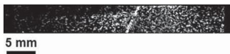
Fig. 2. Subtraction of two successive frame images obtained by LST revealing a PLC band in the middle of the tensile specimen; recrystallized sample state (50 mm gauge length).
