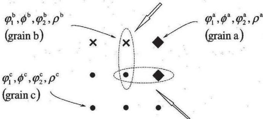
1. calculate probability:  $w^{a-c} = \sigma \left( \frac{m_0^{a-c}}{m_0^{\max}} \right) \left( \frac{p^{a-c}}{p^{\max}} \right) \exp \left( - \frac{(Q_{gb}^{a-c} (\Delta g_{a-c}, n_{a-c}) - Q_{gb}^{\min})}{k_B T} \right)$
