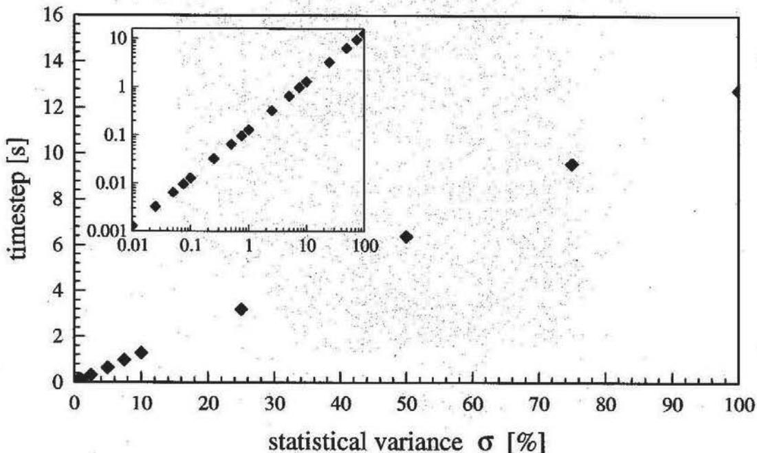
Figure 4. Linear relation between the time constant  $\Delta t$  of the simulation and the statistical variance  $\sigma$  of the Monte Carlo integration method according to equation (10). The characteristic time scale  $\Delta t$  of the simulation is  $1/\nu_0^{\min}$ . The inset shows the linear relation for small time steps.
