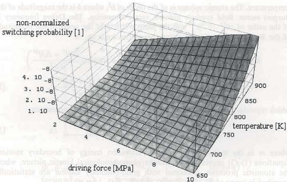
Figure 2. Plot of the non-normalized probability factor  $(p\Omega)/(k_B T) \exp(-Q_{gb}/(k_B T))$  as a function of absolute temperature and driving force for an average aluminium large-angle grain boundary with an activation energy of the mobility of  $Q_{gb} = 1$  eV. The probability factor represents the linearized and the nonlinearized part of the Boltzmann terms in equations (1) and (2).
