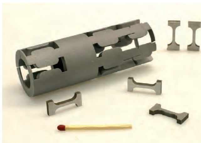
Fig. 3: Miniature tensile creep specimens taken from a tempered martensite ferritic steel tube.
