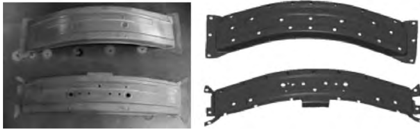
Figure 10.14 Stamping part of a car boot. Photographs and visualized measured data. After stamping and after trimming.
