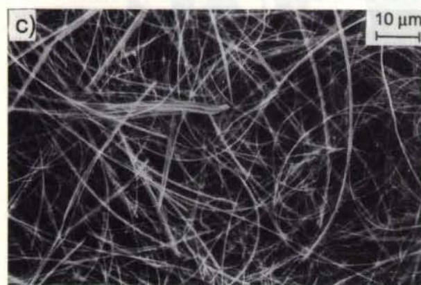
Fig. 11a to c. SEM micrographs of Nb filaments, isolated by dissolving the Cu matrix at different degrees of wire deformation, a) \epsilon = 88.9\% , b) \epsilon = 94.8\% , c) \epsilon = 99.995\% .
