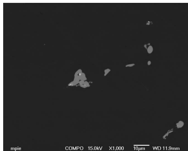
Fig. 1. SEM micrograph of the investigated alloy after the 4 h heat treatment at 1200 °C.
