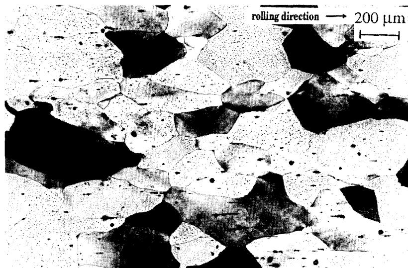
Fig. 9. Longitudinal section of the material after casting, thermomechanical hot rolling and subsequent annealing at 870 K.
