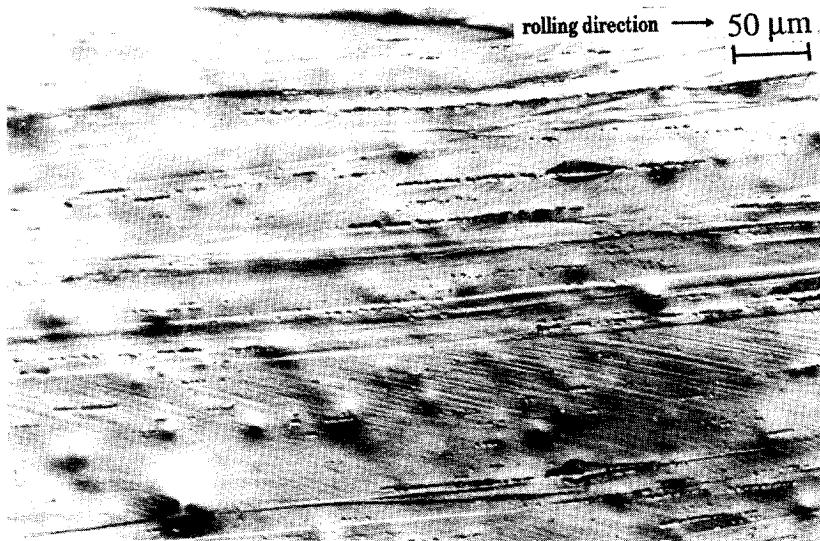
Fig. 11. Longitudinal section of an 80% rolled specimen ( $T_{\text{roll}} = 800\text{--}830\text{ K}$ ). In numerous grains straight slip lines were observed.
