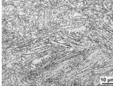
A micrograph showing a more extensive and larger precipitate structure than at 60min. A scale bar indicates 10 μm.<br>10 μm                                                                               |
