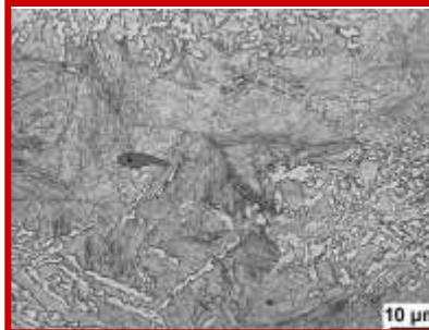
A micrograph showing a significantly coarser precipitate structure compared to the no deformation cases. A red box highlights a specific area for closer inspection. A scale bar indicates 10 μm.<br>10 μm |
