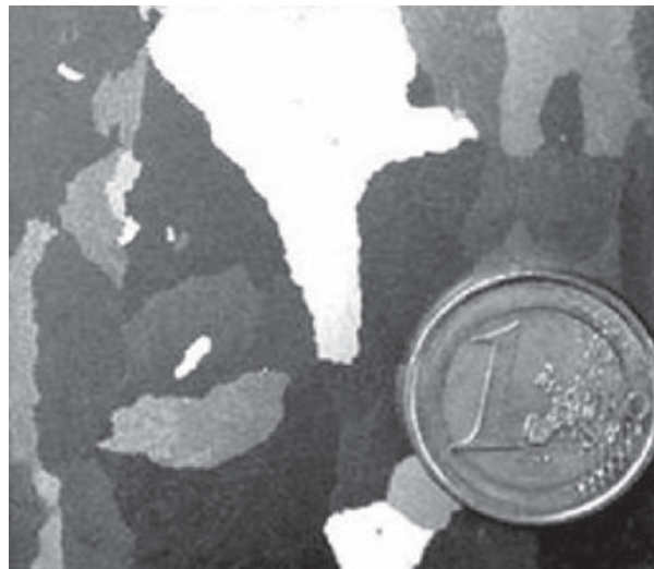
Figure 51 Typical size of Goss grain after abnormal grain growth (Dorner et al., 2006).
