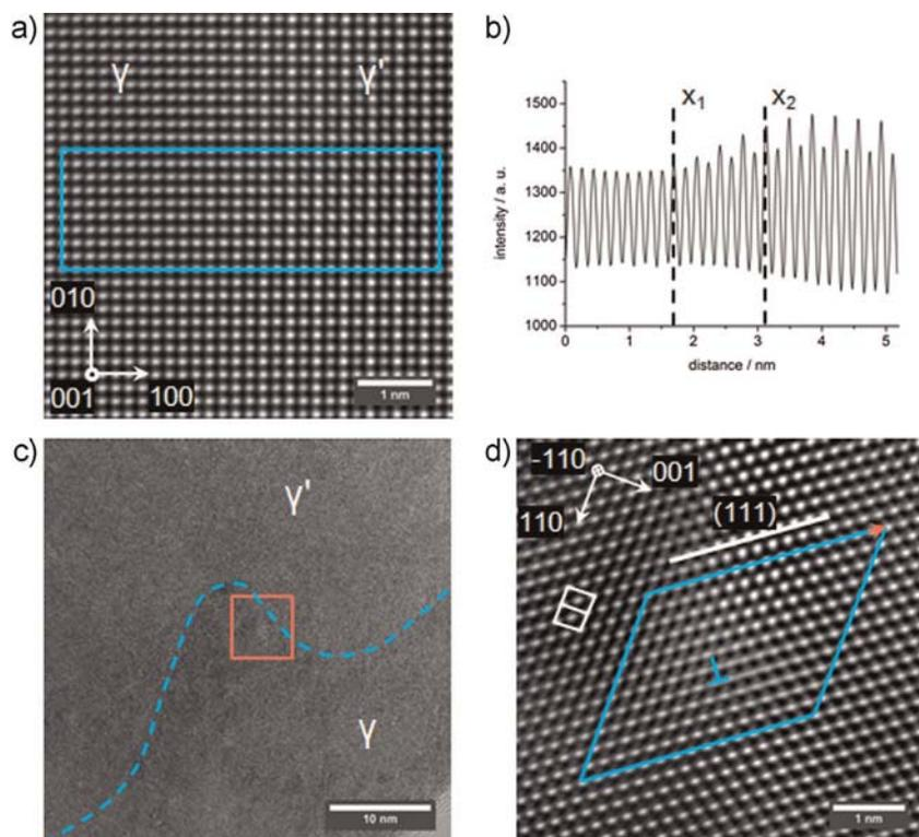
Fig. 10. Microstructural results obtained using HRTEM (FEI Titan<sup>3</sup> 80–300). (a) Fast Fourier transform (FFT) filtered image of a  $\gamma/\gamma'$ -interface prior to creep. (b) Corresponding intensity line profile across the interface. (c) Curved 0.4%  $\gamma/\gamma'$  interface after tensile creep. For details see text. (d) HRTEM image showing an extra half plane associated with a  $60^\circ$  interface dislocation.
