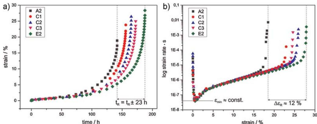
Fig. 9. Miniature specimen creep data from five reference locations A2, C1–C3, and E2 from Figure 2b. Stress and temperature: 160 MPa and 1323 K, respectively. (a) Strain versus time. (b) Strain rate versus strain in a log-linear plot.
