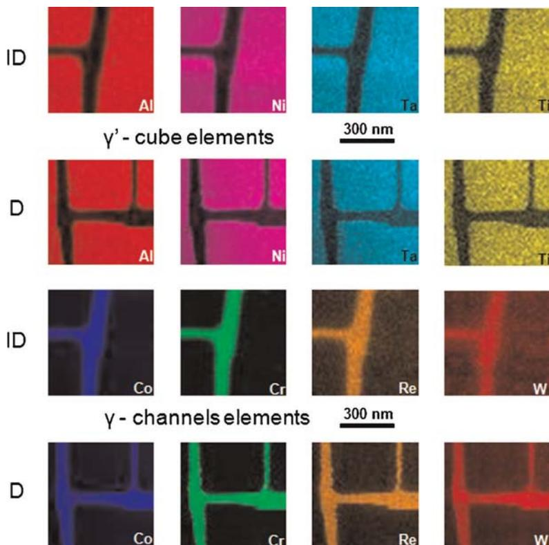
Fig. 7. Series of EDX maps obtained using TEM, showing the partitioning of Al, Co, Cr, Ni, Re, Ta, Ti, and W in our single crystal superalloy. (a) Alloy elements, which partition to  $\gamma'$  (upper row – interdendritic region, lower row – dendrite core). (b) Alloy elements, which partition to  $\gamma$  (upper row – interdendritic region, lower row – dendrite core).
