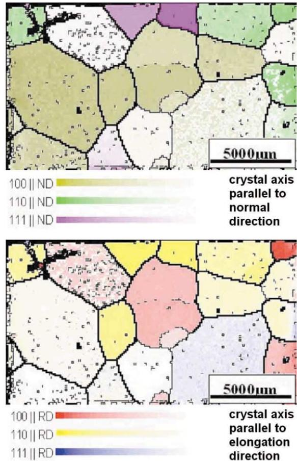
Fig. 5. Crystallographic microtexture of the sample before plastic deformation using separate color scales for the crystallographic axes parallel to the direction normal to the compression axis (ND) and parallel to the extension direction (RD). The grain boundaries with orientation changes above 15° were superimposed in Fig. 6.
