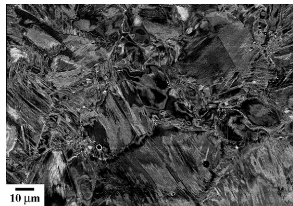
Fig. 8. Large view field ECCI image of deformed sample to 0.3 true strain/1150 MPa showing a multiple twin structure with dislocation substructures.
