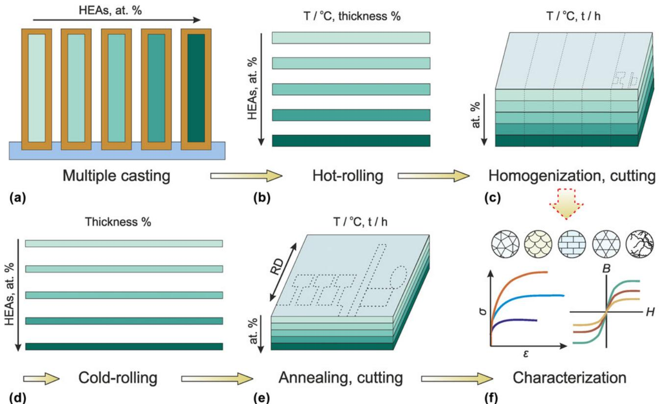
FIG. 2. Schematic sketches illustrating the RAP approach for combinatorial synthesis and processing of HEAs. (a) Multiple casting; (b) hot-rolling; (c) homogenization and cutting; (d) cold-rolling; (e) annealing and cutting; (f) characterization. The RAP approach can also be applied to many other material systems including advanced high-strength steels.<sup>18</sup>
