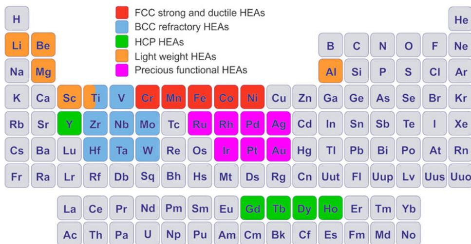
FIG. 1. Element groupings highlighting the main ingredients used to synthesize alloys pertaining to the five most typical HEA families, i.e., FCC-based strong and ductile HEAs, BCC-based refractory HEAs, HCP structured HEAs, light weight HEAs, and precious functional HEAs. For simplicity, other HEA systems or variants of the alloy classes mentioned above including other substitutional elements or interstitial ones such as B, C, N, O, etc. are not color-coded here.
