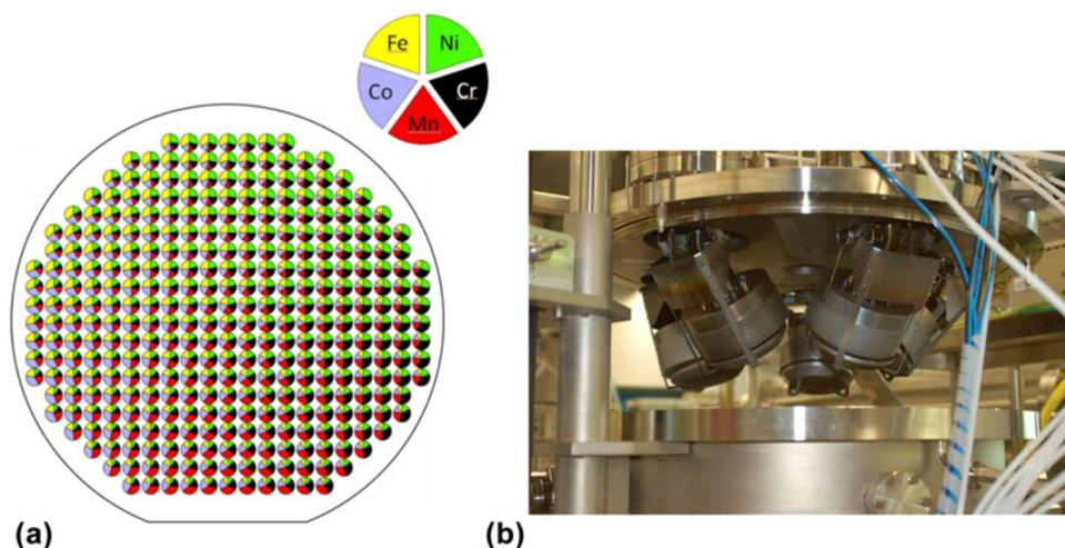
FIG. 8. (a) Visualization of the quinary compositions contained in an exemplary thin-film library of Cr-Mn-Fe-Co-Ni co-sputtered from individual single-element targets, indicating the relative concentrations at each of 342 EDS measurement points. Legend identifies the elements and respective cathode positions. (b) Opened co-sputter chamber showing 5 confocal, 100 mm diameter magnetron sputter cathodes.
