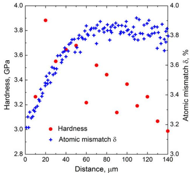
FIG. 5. Direct comparison of microhardness and atomic mismatch  $\delta$  (the mean square deviation of the atomic size of elements<sup>47</sup>) in a section of a diffusion region in a Co–Cr–Fe–Mn–Ni quinary diffusion multiple made of  $\text{Fe}_{50}\text{Mn}_{50}$ ,  $\text{Co}_{50}\text{Ni}_{50}$ , and Ni. Data points are mainly taken from Ref. 22.
