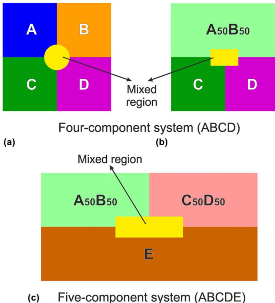
FIG. 4. Schematic sketches showing some examples of diffusion-multiple setups for combinatorial HEA research. (a and b) Two typical setups for four-component alloy systems. (c) A typical setup for five-component HEA systems.<sup>21,22</sup>
