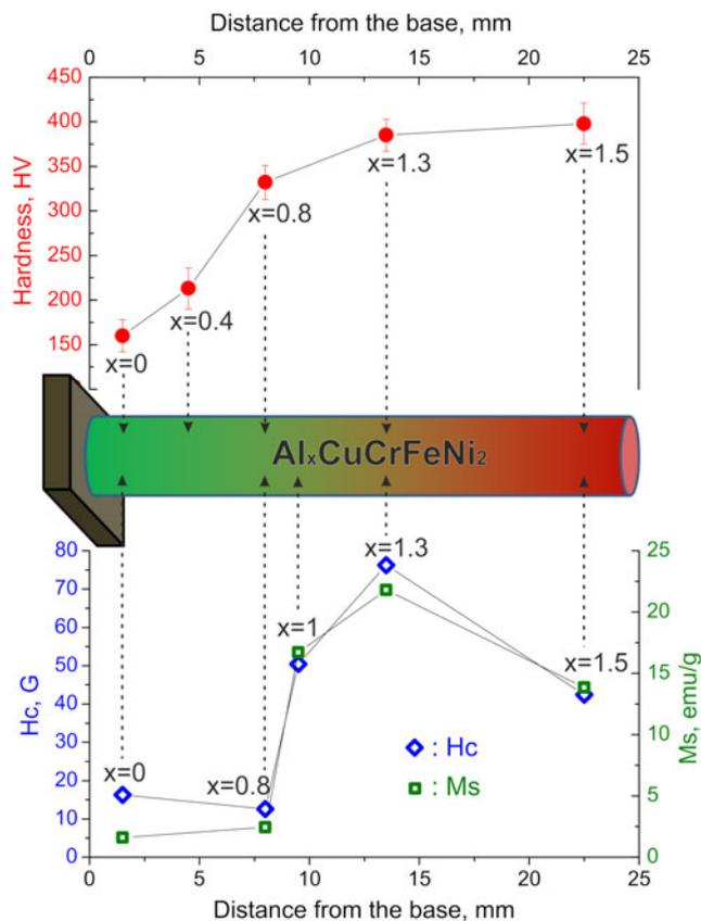
FIG. 7. Microhardness values and magnetic properties along the length direction of the compositionally graded  $\text{Al}_x\text{CrCuFeNi}_2$  ( $0 < x < 1.5$ ) HEAs produced by laser deposition. The compositional gradient has a length of  $\sim 25$  mm. Ms and Hc refer to saturation magnetization and coercivity, respectively. Data points are mainly taken from Ref. 23.
