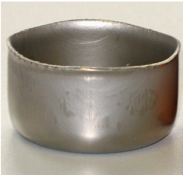
Fig. 10. Experimentally drawn cup of the ferritic stainless steel X6Cr17.
