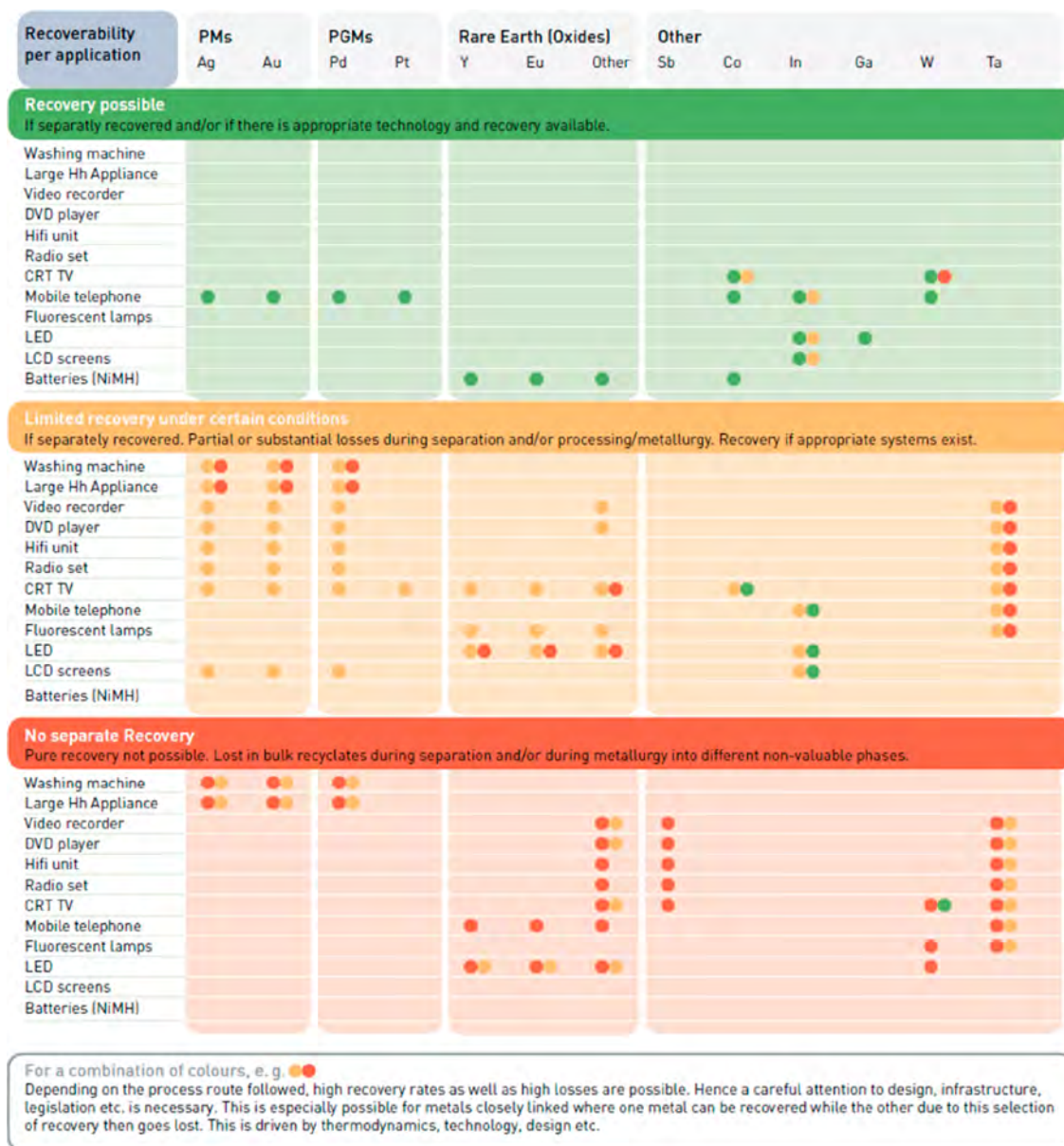
Figure 34. Metals that can be recycled from several types of products and metals that are hard to recover. 156 The figure is reproduced with permission from ref 156. Copyright 2013, UN Environment Programme UNEP.
