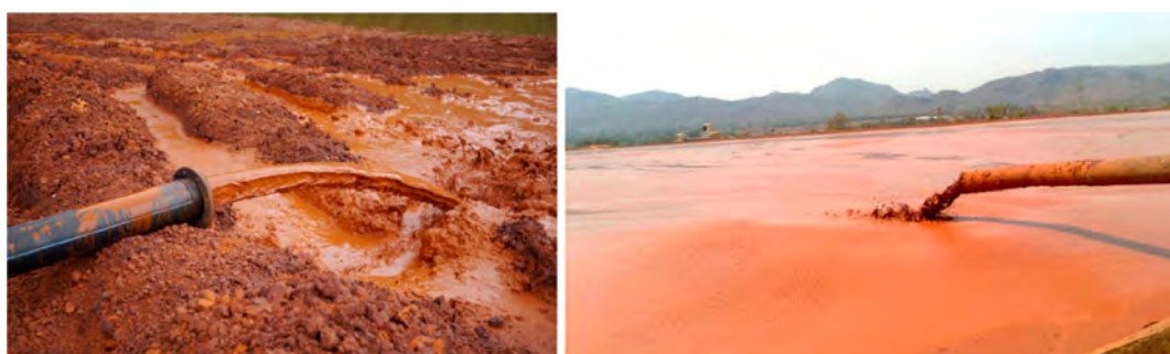
Figure 78. View at typical red mud dump sites. Red mud is a bauxite residue, rich in iron oxide and titanium oxide as well as in a few rare earth metals. Bauxite serves as primary feedstock mineral for producing the alumina which is then used subsequently in fused-salt electrolysis to produce metallic aluminum. The red color comes from the high proportion of iron oxide compounds in the bauxite. In the context of developing re-mining opportunities, such dumped residues can become potentially commercially viable feedstock sources for future sustainable metallurgical production (see sections 6.4.2–6.4.5).
