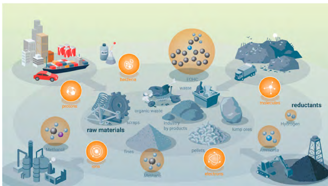
Figure 73. Different possible combinations of metal feedstock (scrap and minerals of different grade and dispersion) and reduction pathways in different aggregate states. The overview shows some of the currently emerging opportunities for basic research for the case of iron making, considering the origin of the feedstock, coming for instance from primary resources (mining), secondary resources (scrap), or tertiary resources (re-mined material, dumped waste). The latter resources can be both of mineral origin (e.g., red mud, as metal carrier) or of biological origin (biomass, as reductant).
