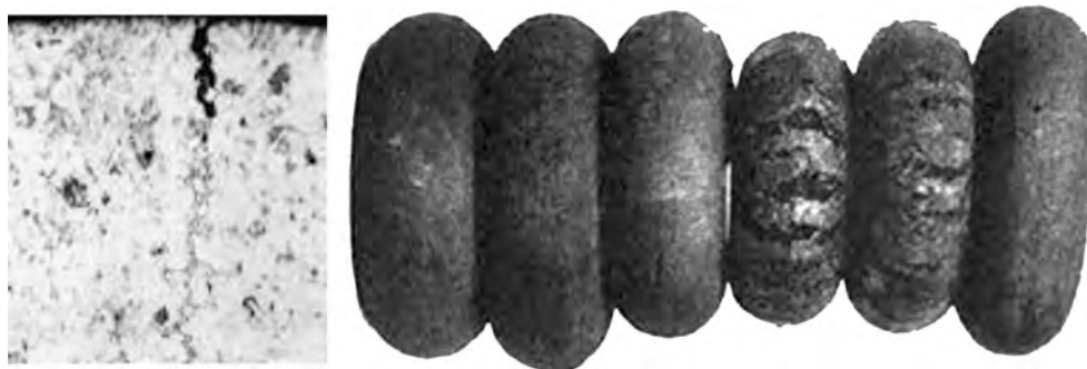
Figure 103. Increased amounts of copper, tin and lead in steels can lead to liquid-metal embrittlement through the formation of low-melting eutectics on decorated grain boundaries. The image shows a specific example of the effects of copper on the embrittlement of steel. 413 The figure is reproduced with permission from ref 413. Copyright 1931, Verlag Stahleisen GmbH.
