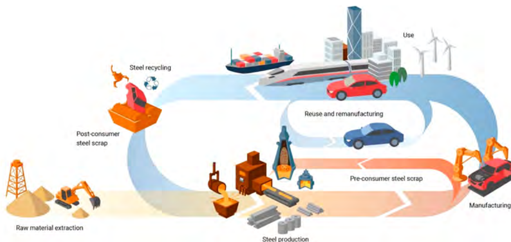
Figure 11. Some streams for old scrap (contaminated post-consumer scrap) and new scrap (runaround and in-production scrap with certified chemical composition), shown here for the case of steel.
