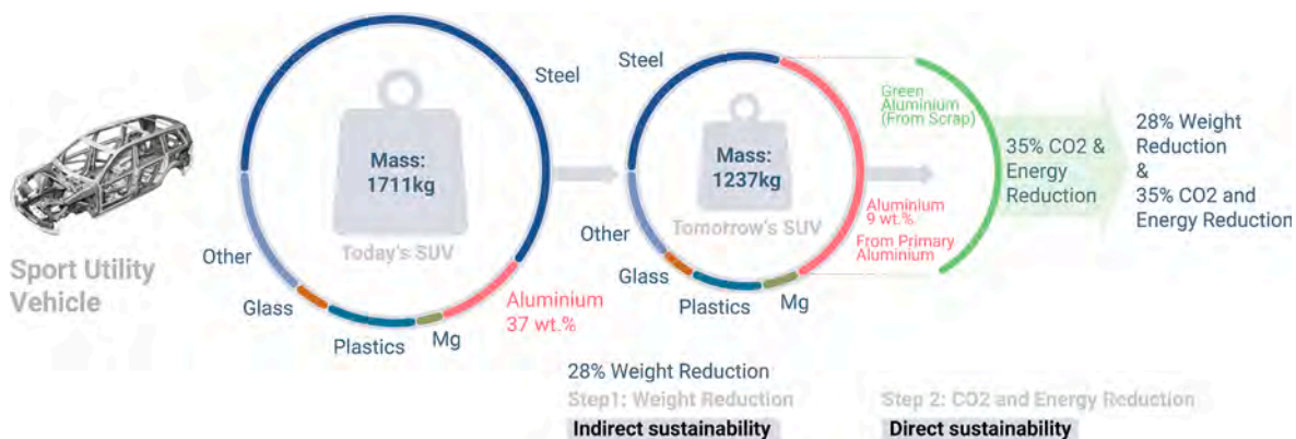
Fig. 6. Example revealing the dual effect of aluminum alloys made from scrap: weight reduction and the associated fuel savings (left) plus reduction in energy consumption and GHG output from synthesis when using alloys made from scrap (right). Step 1 (data from AI Association) shows how much mass is saved when increasing Al from 9 to 37 wt%. Step 2 shows that this generates a 28% reduction in mass plus a 35% reduction in energy consumption and GHG emission when using scrap-based Al.
