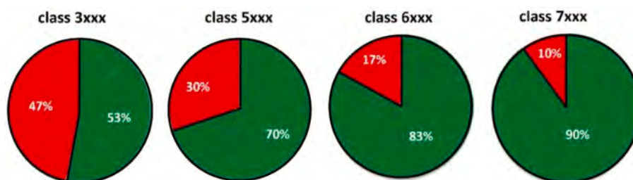
Fig. 46. Machine-learning-based classification findings for mixed aluminum scrap chips, probed by considering the chips' LIBS spectra. Classification of these measurements into aluminum alloy groups proceeded by using a modified artificial neural network. Green: correct; red: incorrect. Figure used with permission from [769]. (For interpretation of the references to color in this figure legend, the reader is referred to the web version of this article.)
