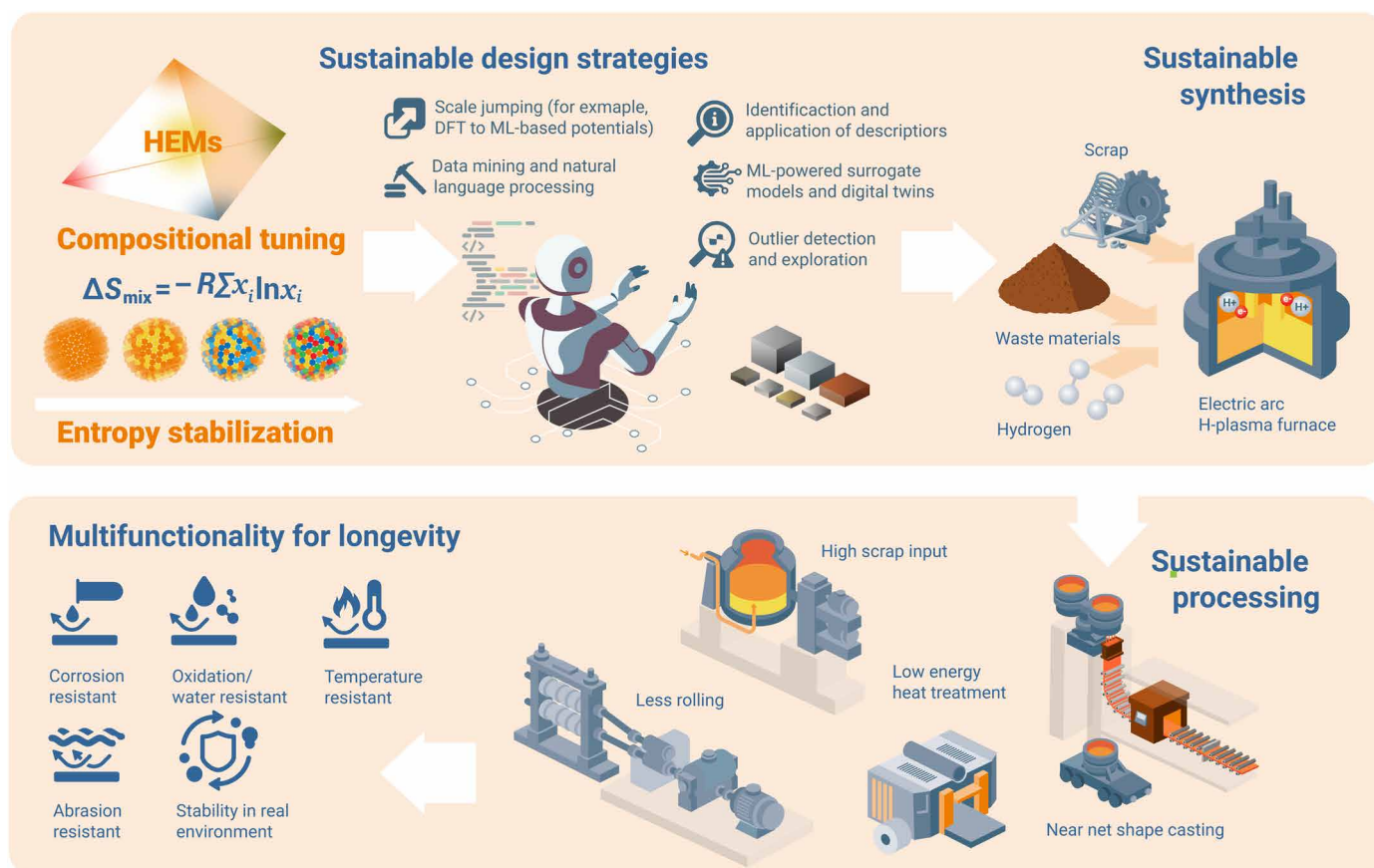
Fig. 6. Sustainable design and manufacturing strategies. Different measures have to be taken into account in the design, synthesis, and processing of mass-produced HEMs to reduce energy consumption and CO 2 emissions and ensure multifunctionality and longevity.
